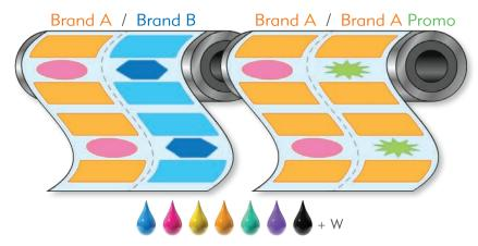
**Xcolor™ Extended Gamut Process** means greater flexibility and potential cost savings, by reducing the number of print stations and allowing for ganged runs.
